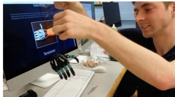
Figure 3 Students learn how to attach tension strings that add functionality to the device. In this iteration they used glow in the dark filament to provide another option to our community partner.
