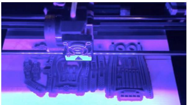
*Fig. 5 A 3D printer makes parts for a prototype of a prosthetic hand.*
