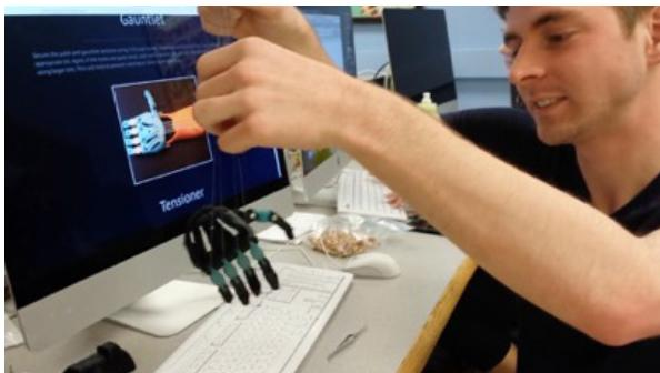
Figure 3 Students learn how to attach tension strings that add functionality to the device. In this iteration they used glow in the dark filament to provide another option to our community partner.
